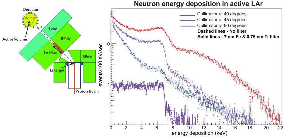
Without filtering near-threshold reaction combined with angular tuning can produce a 'shoulder' but multiple scattering and detector response make this undesirable
