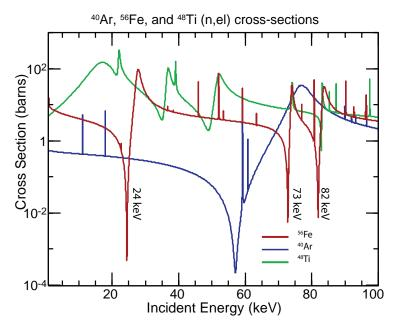
The 73 keV notch in <sup>56</sup>Fe was selected to target the lower energy portion of the (n,el) resonance in <sup>40</sup>Ar
