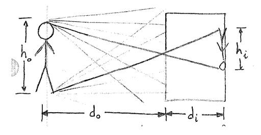
Pinhole camera: Pro: image infinitely sharp Con: infinitely inefficient
