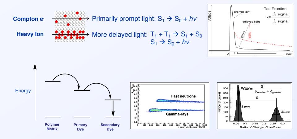
The PSD technique exploits difference in time characteristics in signals induced by heavy ions (recoil protons) and Compton electrons
