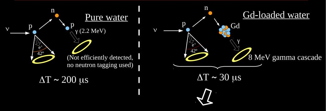
With tight time (delayed) and position coincidence between positron and neutron capture (90% neutron capture on Gd with 0.2%  $Gd_2(SO_4)_3$ concentration) we will be able to tag neutrons with high efficiency
