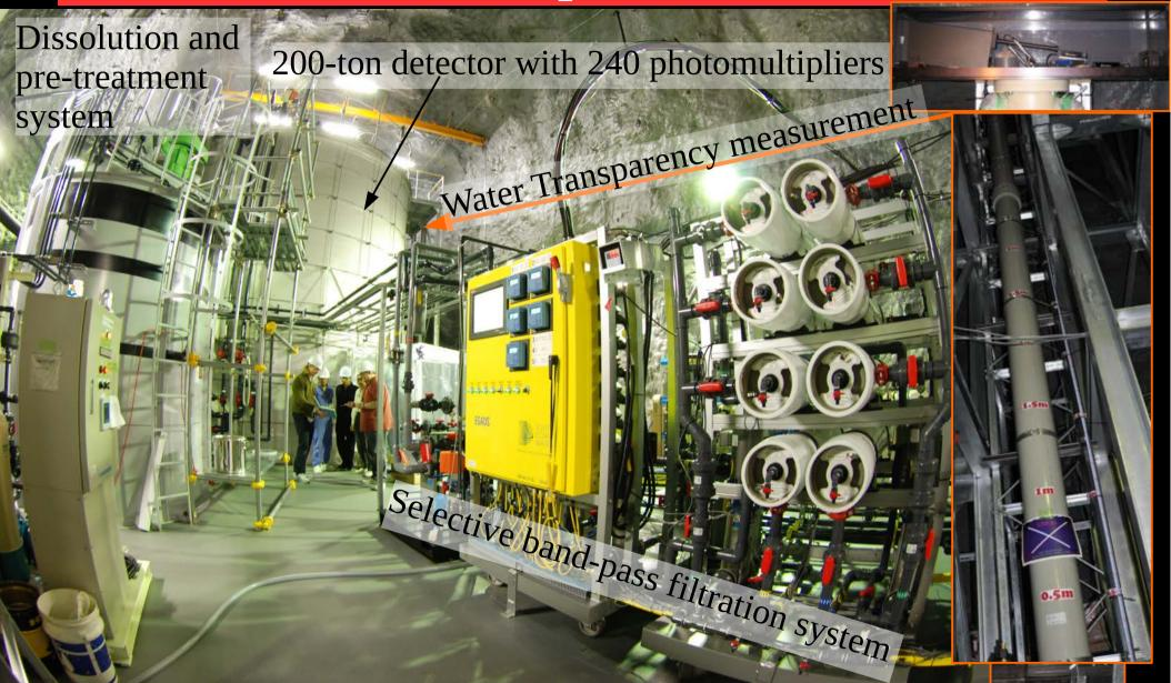
The EGADS detector was build using the same materials as in SuperK
