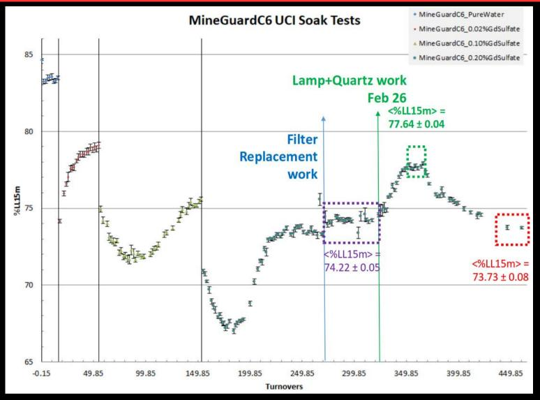
Soaked Mine-guard-C in Gd loaded water with good results: Cherenkov ilght loss in 15 m is 77.64 % (well within the typical SK-III SK-IV values)
